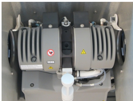
Figure 9. Graphite furnace assembly. The transversely heated tube is located at the center of the figure (black), with electrode contacts above and below. The grey cylindrical structure is a water cooled jacket, also enclosing an electromagnet used in Zeeman noise correction. The tubes at top right and left supply cooling water, while the lines at bottom supply argon both internal and external to the tube.
