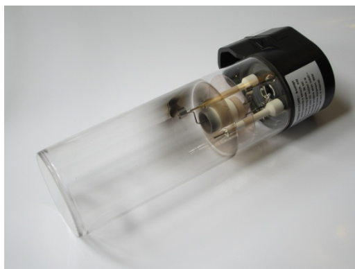
Figure 5. A typical hollow cathode lamp. The cathode is at the center, the cylindrical shape of which helps direct the emitted radiation towards the end of the tube, most often a quartz window. Dual anodes are located on either side of the cathode.
