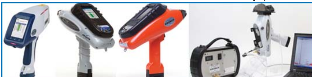
Figure 1. Examples of field-portable XRF instruments. Taken from: http://www.bruker-axs.com/handheldx-rayspectrometry.html
