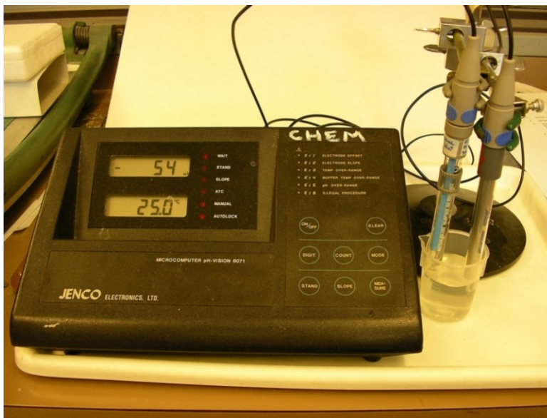
Figure 1. An experimental setup for the direct potentiometric measurement of sodium ion in aqueous solution.
