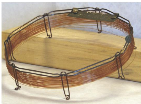
Figure 5. Typical example of a capillary column for gas chromatography. This column is 30 m long, has an internal diameter of 247 \mu\text{m} , and has a 0.25 \mu\text{m} coating of liquid stationary phase on its interior surface. From Figure 12.4.3 in David Harvey, Analytical Chemistry 2.1 , licensed under CC BY-NC-SA 4.0.
