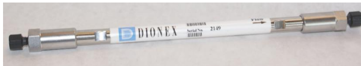
Figure 6. Typical packed column for HPLC. This column has an internal diameter of 4.6 mm, is 150 mm long, and is packed with 5 \mu\text{m} particles coated with stationary phase. From Figure 12.5.2 in David Harvey, Analytical Chemistry 2.1 , licensed under CC BY-NC-SA 4.0.
